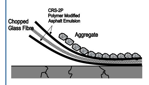
A specially developed unit chops (60-90mm length) glass fibers in-place and sandwiches them between two layers of asphalt emulsion prior to the application of 6.35mm, 9.5mm or 12.5mm size aggregate, combinations thereof, which is then rolled into the surface. The glass fibers are applied at a rate of approximately 70g per m2, depending on the severity of the cracking, and the asphalt emulsion is applied in two simultaneous applications totaling 1.8 to 2.7 litres/m2.
