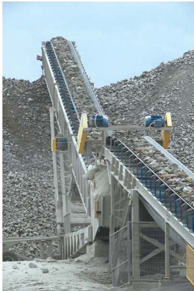
Product from the crusher is sent to the surge pile via a 54 in. x 150 ft. Masaba radial stacker.
