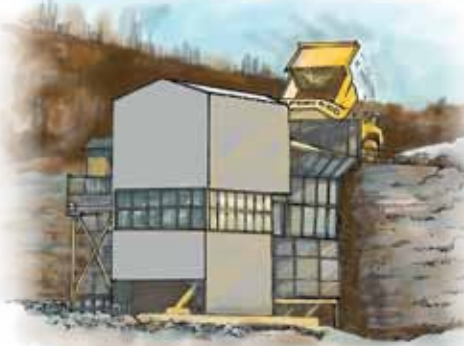
haul truck dumps into the enclosed primary crusher
