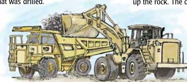
Haul truck is filled by a face loader at the muck pile.
