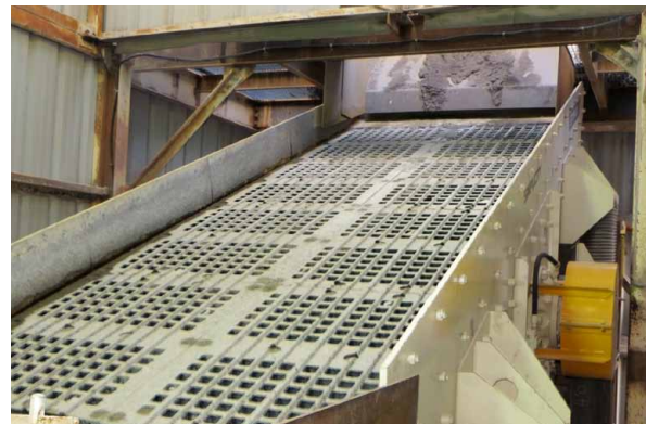
Rubber decking has replaced metal screen decking on the conveyor belt leading to the secondary crushing plant.
